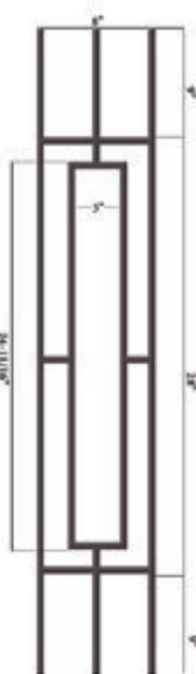
HF 9.4.11 Ends: 1/2" Sq. Height: 46" Wt. 4.5 lbs. TUBULAR (Rake)
