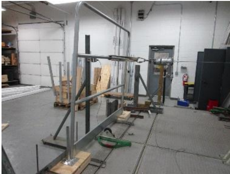
Photo No. 3 Concentrated Horizontal Load at Mid-Span of Mid Rail
