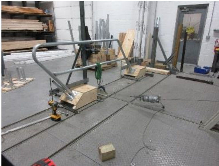
Photo No. 4 Concentrated Vertical Load at Mid-Span of Mid Rail
