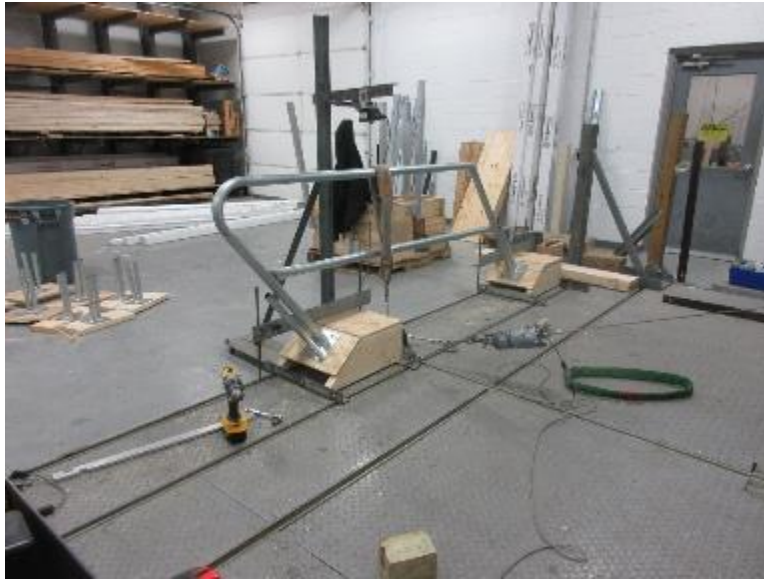
Photo No. 2 Concentrated Vertical Load at Mid-Span of Top Rail
