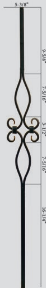
HF 16.8.9 Ends : 5/8" Sq. Height: 44" Wt. 4 lbs. TUBULAR
