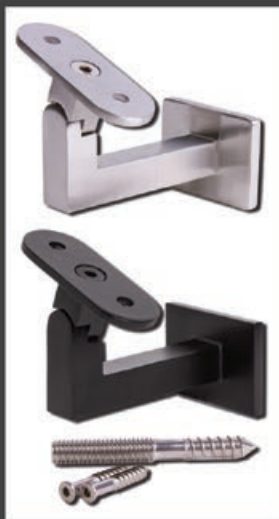
HF17.4002 Stainless Steel(304) HT. 2-1/2" Base = 1-1/2" x 2" Extends 3-1/4" off wall ADJUSTABLE
