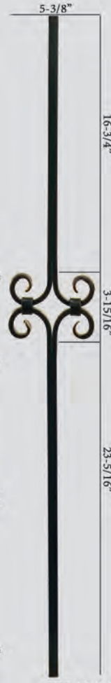
HF 16.8.8 Ends : 5/8" Sq. Height: 44" Wt. 3 lbs. TUBULAR
