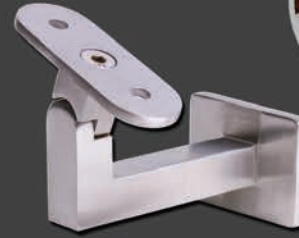
HF17.4002 HT. 2-1/2" Base = 1-1/2" x 2" Extends 3-1/4" off wall ADJUSTABLE
